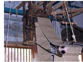
Punched card loom mechanism in silk-weaving workshop; Varanasi, Uttar Pradesh, India
