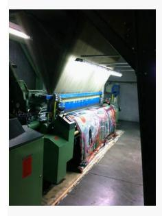
Small metal shuttles flew back and forth with the weft threads, woven patterns emerging at about an inch every minute. Rows and pallets of thread of every color were stacked on warehouse racks around the room.
