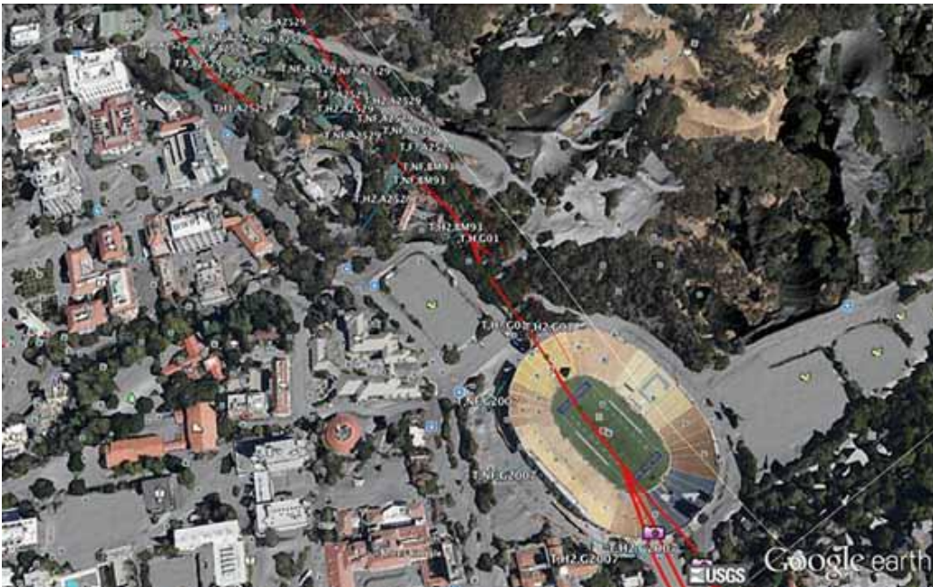
The Hayward Fault trace superimposed onto a map of the University of California, Berkeley, campus, as seen in the USGS Hayward Fault Virtual Tour
